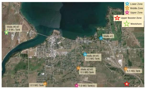
The wells have a total pumping capacity of 1870 gpm (gallons per minute). The Department of Environmental Quality (DEQ) requires a water system to supply the maximum daily demand for water with the largest well out of production. Polson currently meets this requirement.
